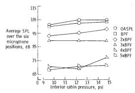
Fig. 9 Effects of cabin pressure on space averaged sound pressure levels for the treated airplane.
