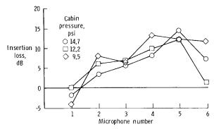
Fig. 6 Spatial variation of the insertion loss at  $2 \times BPF$  (210 Hz) for three cabin pressures.
