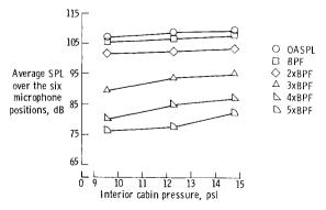
Fig. 8 Effects of cabin pressure on space averaged sound pressure levels for the "green" airplane.
