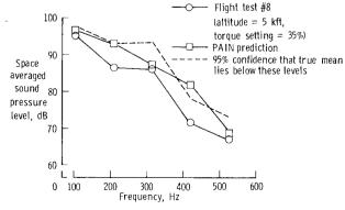
Fig. 12 Measured and predicted space averaged sound pressure levels (treated airplane, 35% low engine torque).
