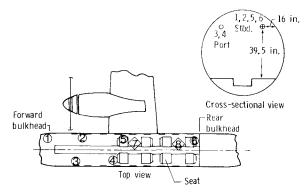
Fig. 1 Microphone locations relative to the interior plan of the treated airplane.
