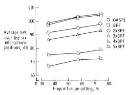
Fig. 10 Effects of engine torque on space averaged sound pressure levels for the treated airplane.
