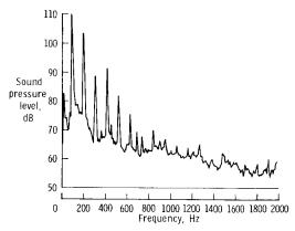
Fig. 3 Narrowband analysis at microphone 2 for the flight conditions of run 1 ("green" airplane).
