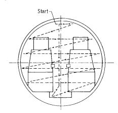
Fig. 2 Microphone sweep path for hand-swept interior noise measurements at locations 7 and 8.
