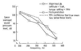
Fig. 11 Measured and predicted space averaged sound pressure levels (treated airplane, 74% high engine torque).
